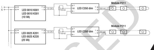
LED modules must be wired in series connection to the constant current source Control C350 dim
