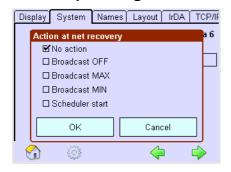
In the Configuration menu it can be defined how the x-touchBOX/PANEL will behave after a power failure.
