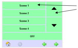
In software version 3.00 the commands of the scene- and the dim-buttons are configurable. (See operation manual section:
